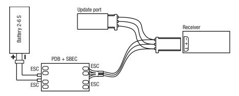
The small 3 poles socket is provided for switch functions. See paragraph "Programming the user setup"
